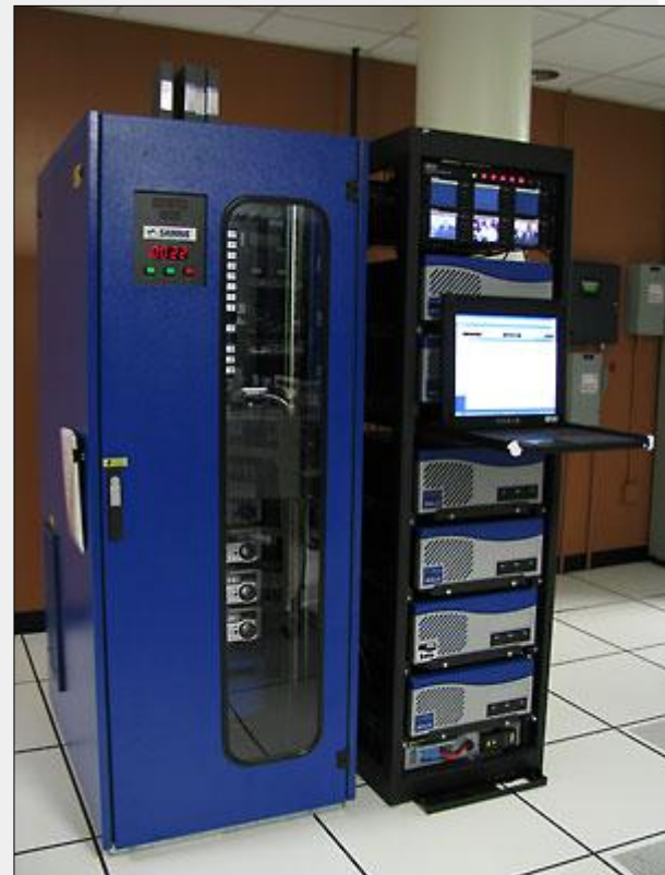
One of the robots used to import the video tapes to the server for digital processing
