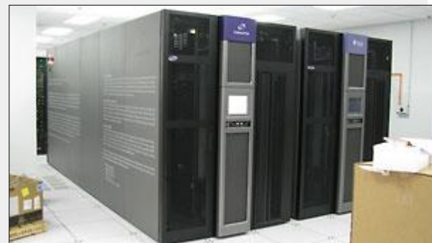
After the master tapes are digitized, the resulting Motion JPEG2000 files will be stored on the two Sun Storagetek servers pictured here. The digital files will also allow for easier access to the testimonies by students, researchers, and scholars worldwide.
